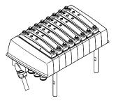
The signals are transmitted from the controller to the valve terminal via a pre-assembled or self-assembled multi-wire cable to the multi-pin plug connection, which substantially reduces installation time. The valve terminal can be equipped with max. 32 solenoid coils. This corresponds to 2 to 32 valves. The multi-pin cable should be no longer than 30 m.
