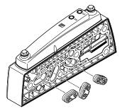
The MPA-C offers a number of options for creating pressure zones if different working pressures are required. Duct 1 and/or duct 3 and/or duct 5 are interrupted by inserting a separator in the sub-base. Every pressure zone must have its own supply. The following supply options are available:
