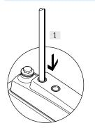
[1] Press in the plunger of the MO with a blunt plastic pin. The pilot valve switches and actuates the main valve.
