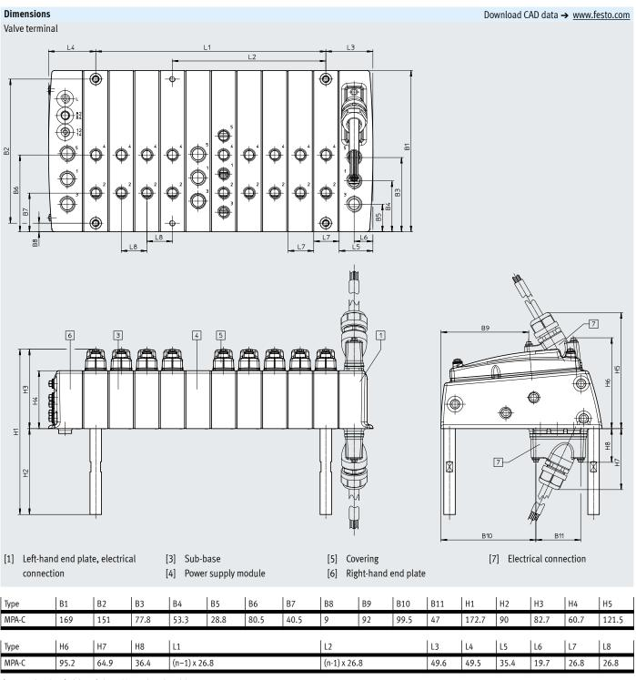
1) n = total number of sub-bases/valve positions and supply modules
