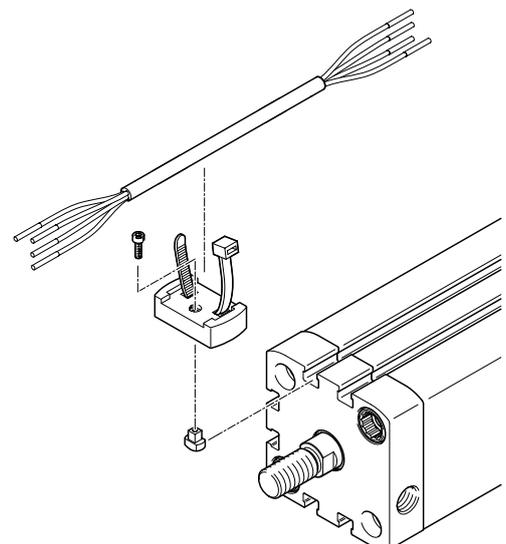
The mounting kit guarantees secure mounting in T-slots from Festo. The geometry of the retaining bracket and of the slot nut are precisely adapted to these T-slots.
