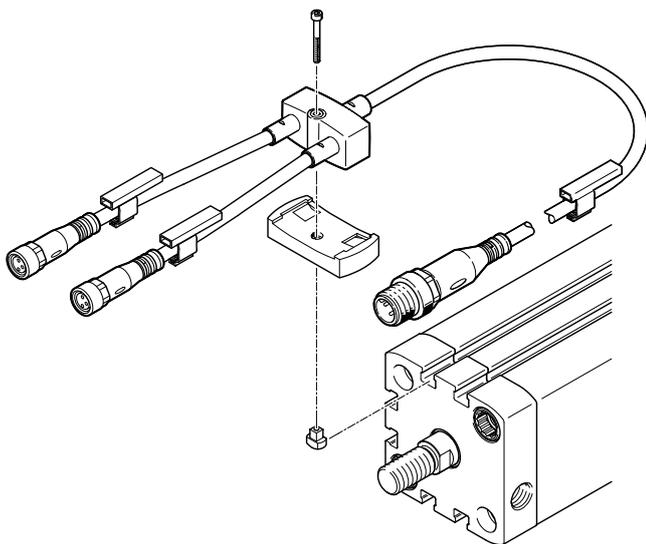
The distributors NEDY have a through-hole suitable for an M2 screw on the distributor housing. The mounting kit is available in two sizes for mounting in T-slots.
