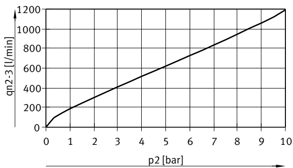
Flow rate q_n from 2 -> 3 as a function of excess output pressure p_2 , VPPM-6L/F-...-0L10H-... (10 bar)
