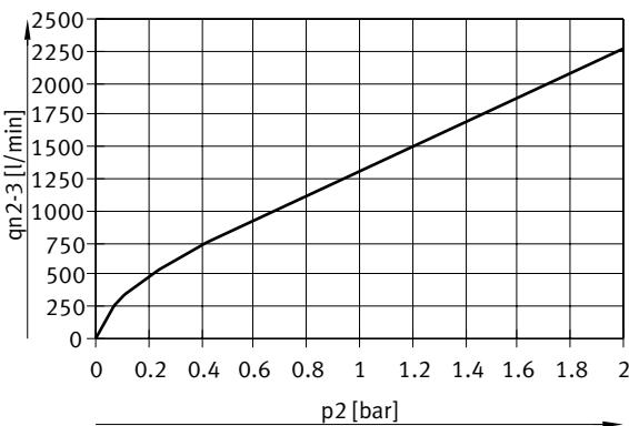
Flow rate  $q_n$  from 2 → 3 as a function of excess output pressure  $p_2$ , VPPM-12L...-0L6H... (8 bar)
