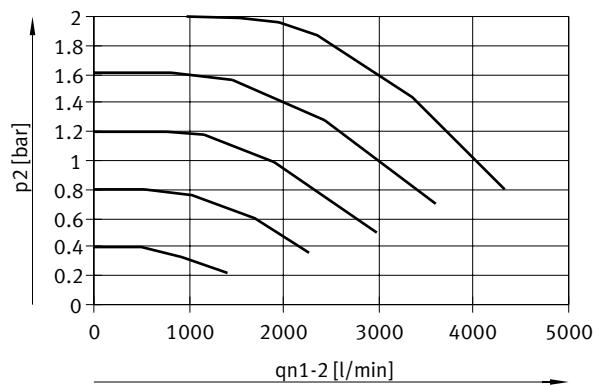
Flow rate  $q_n$  from 1  $\rightarrow$  2 as a function of excess output pressure  $p_2$ , VPPM-12L-...-0L6H-... (8 bar)
