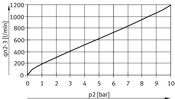
Flow rate  $q_n$  from 1  $\rightarrow$  2 as a function of excess output pressure  $p_2$ , VPPM-8L/F...-0L2H... (2 bar)
