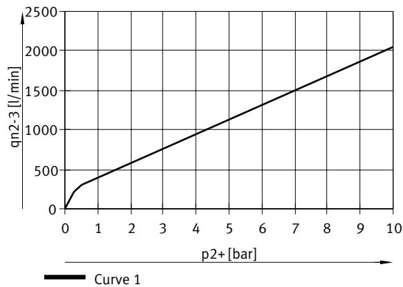
Flow rate  $q_n$  from 1  $\rightarrow$  2 as a function of excess output pressure  $p_2$ , VPPM-12L-...-0L2H-... (4 bar)
