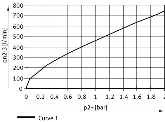
Flow rate  $q_n$  from 2 -> 3 as a function of excess output pressure  $p_2$ , VPPM-8L/F-...-OL6H-... (6 bar)
