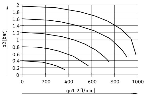
Flow rate  $q_n$  from 1  $\rightarrow$  2 as a function of excess output pressure  $p_2$ , VPPM-8L/F...-0L6H... (6 bar)
