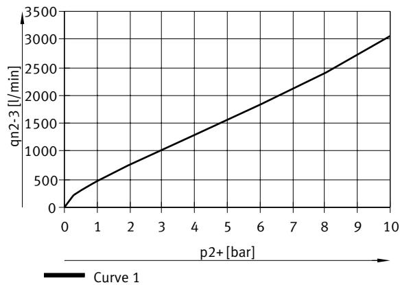
Flow rate  $q_n$  from 1 → 2 as a function of excess output pressure  $p_2$ , VPPM-8F/8TA...-0L2H... (2 bar)
