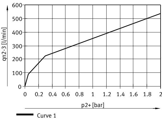
Flow rate  $q_n$  from 2 -> 3 as a function of excess output pressure  $p_2$ , VPPM-8F/8TA-...-OL6H-... (6 bar)
