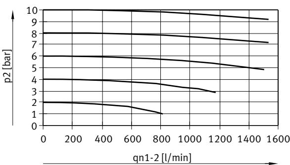
Flow rate  $q_{n2}$  from 2 → 3 as a function of excess output pressure  $p_2$ , VPPM-6L/F-...-0L2H-... (2 bar)
