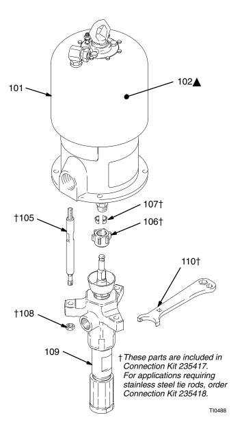
Part No. 236460 Pump, Series B 68:1 Ratio, with Reduced Icing **Quiet King Air Motor**
