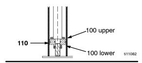
**NOTE:** Whenever you service the lift-rod piston or the guide sleeve, always install new o-rings.
