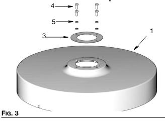
3. Place drum cover (1) on drum (a). For 120 pound models only, tighten thumb screws (6) securely) (Fig. 3).
