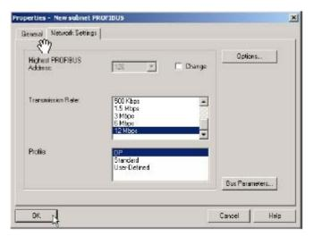
Fig. 56: Set Transmission Rate
