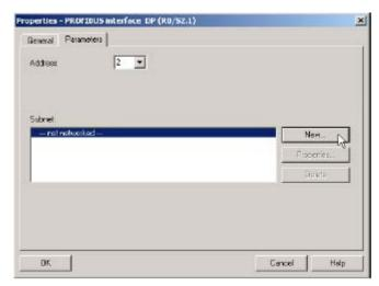
Fig. 55: Create a New Profibus Network
