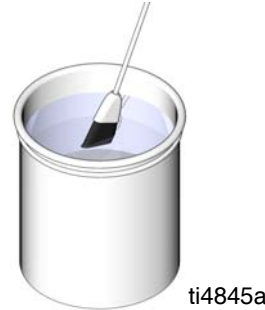
FIG. 15: Use solvent-dipped soft-bristle brush
