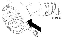
8. Slide pulley onto short axle.
