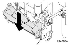
5. Slide single pulley over long axle.
