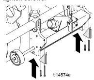
Slide double bead box down through slots on angular brackets and lock into place.
