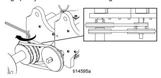
11. Attach pulley guard and tighten two screws.
