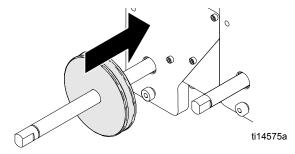
6. Slide bead dispenser engagement wheel pulley onto long axle.
