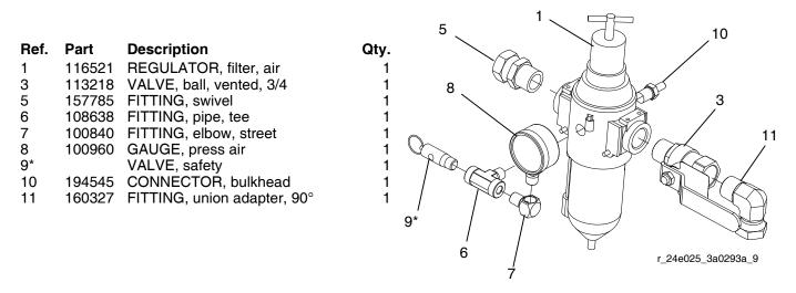
\* Not included with air controls. Replace with appropriate part number from table below according to pump ratio.
