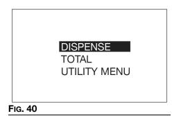
When the MAIN MENU Screen shown in Fig. 40 displays, the meter is ready to use.
