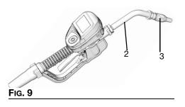
2. With an open-end adjustable wrench on the flats of the nozzle bushing, tighten firmly (Fig. 10).
