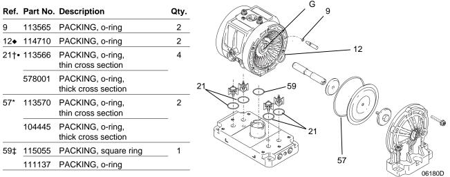
† Use 113566 for series A to E pumps. Use 578001 for series F, G, and H pumps.
