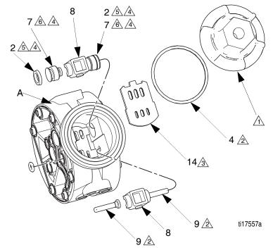
NOTE: Center housing (A) is shown separated from the air covers, but it is not necessary to remove the air covers for this service. Leave the center housing and air covers assembled for this service.
