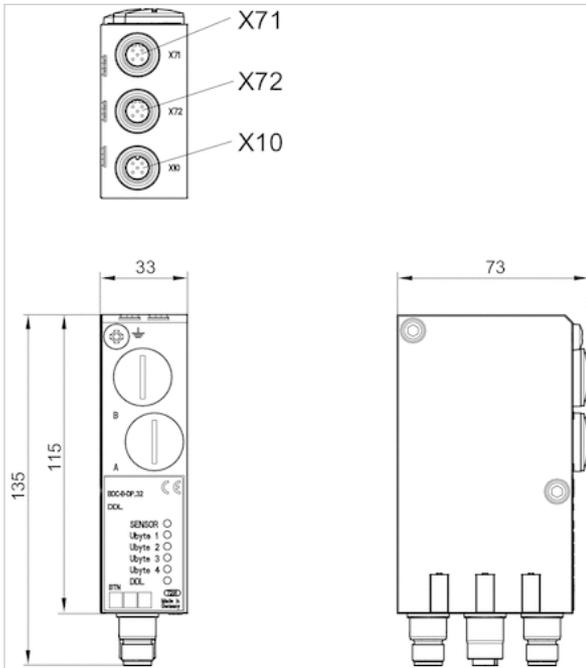
X71 = Bus INX72 = Bus OUTX10 = Spannungsversorgung
