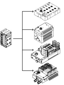
The CPX CTEL master provides 4 external I-Port interfaces, each of which can be connected with a device. I-Port is an interface for exchanging serial data for connecting decentralised modules or valve terminals from Festo. The I-Port interface is based on IO-Link and is compatible with it in certain areas. The connection type corresponds to a star topology. In other words, only one module or valve terminal can be connected to each I-Port. The limitations with respect to IO-Link include:
