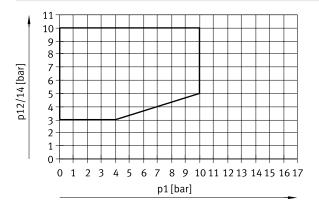
5/2-way valve and 5/3-way valve, external pilot air supply
