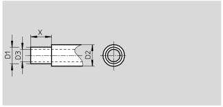
length X. The integrated stop in the PAN-VOS tubing cutter ensures that the sheath is always cut to the correct length X. The blade design prevents damage to the inner polyamide tubing.
