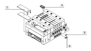
A holder VMPAL-ST-AP-10 (part no. 561109) with inscription labels (part no. 18576, IBS-6x10) can be mounted on each sub-base for labelling the valves.
