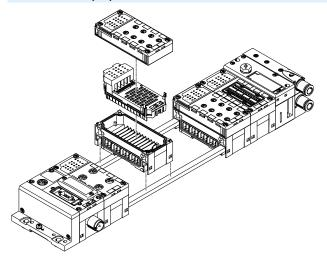
The mechanical connection between the CPX modules is established using tie rods. Two screws in the end plates are all that are needed to assemble the
