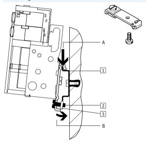
The valve terminal is attached to the H-rail (see arrow A) and then swivelled onto the H-rail and secured in place with the clamping component (see arrow B).
