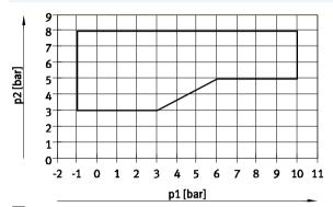
1 Operating range for valves with external pilot air supply
