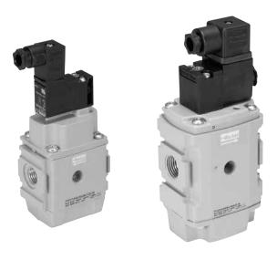
Parker Global Series Combined Soft Start / Dump Valves, provide for the safe introduction of pressure to machines or systems. Soft Start / Dump Valves when set, allow the pressure to gradually build to the set point before fully opening to deliver full flow at line pressure.
