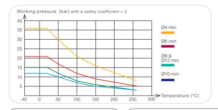
To calculate burst measurements, the values in this graph should be multiplied by 3.
