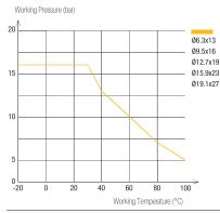
To calculate burst pressure, the values in this graph should be multiplied by 3
