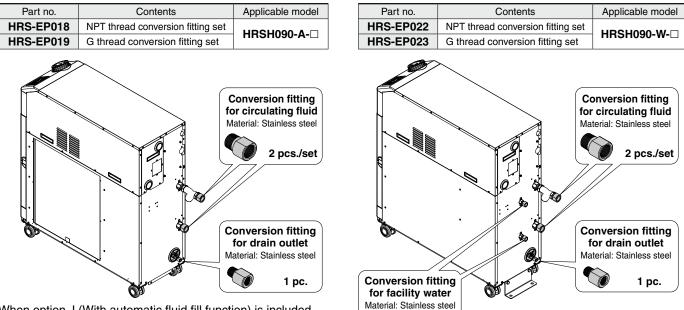
When option J (With automatic fluid fill function) is included, use the following part numbers.
