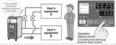
When the product is used with the flow path switched for maintenance, the pressure adjusting function controls the discharge pressure to be stable. (Secure the specified minimum flow for each branch circuit.)
