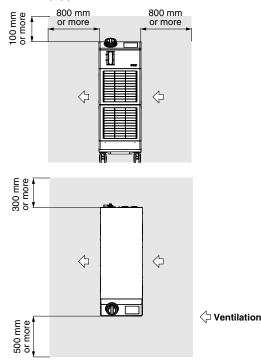
3. If it is impossible to exhaust heat from the installation area indoors, or when the installation area is conditioned, provide a duct for heat exhaustion to the air outlet port of this product for ventilation. Do not mount the inlet of the duct (flange) directly to the air vent of the product, and keep a space larger than the diameter of the duct. Additionally, consider the resistance of the duct when making the air vent port for the duct.
