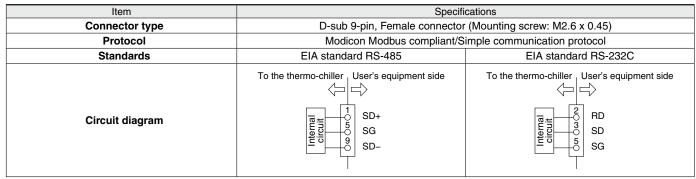
\* The terminal resistance of RS-485 (120 Ω) can be switched by the operation display panel. For details, refer to the Operation Manual, Communication function. Do not connect other than in the way shown above, as it can result in failure.
