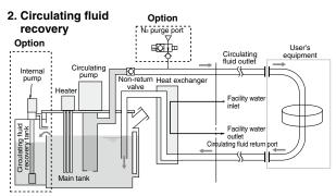
3. Fluid returns to the main tank from the circulating fluid recovery tank.
