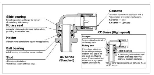
Low torque rotation type Rotary One-touch fittings Applicable to use for oscillating and rotating sections in robots.
