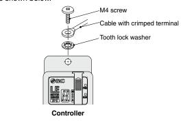
A screws, cable with crimping terminal and tooth lock washer are not included. Be sure to carry out grounding earth in order to ensure the noise tolerance.
