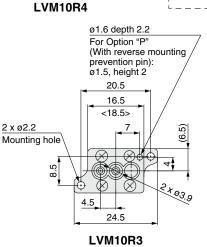
selected as the plate material (wetted parts material "E," "F," or "G"), there is no ø1.6 positioning hole or ø1.5 reverse mounting prevention pin.
