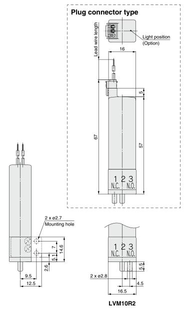
\* The broken lines indicate the model with a bracket.
