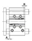
**Auto Switch Proper Mounting Position** Applicable Cylinder Series: MGP
