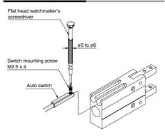
Note) Use a watchmaker's screwdriver with a grip diameter of 5 to 6 mm to tighten the auto switch mounting screw. The tightening torque should be about 0.05 to 0.15 N-m.
