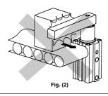
3) Do not clamp during the rotary stroke. Clamp should be performed within the clamp stroke.
