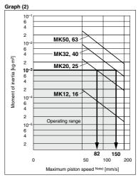
When the arm's moment of inertia is 1 x 10<sup>-3</sup> kg·m<sup>2</sup>, cylinder speed should be MK20/25: 82 mm/s or less,
