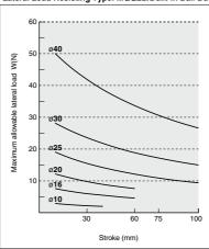
Note 1) The indicated allowable lateral load at the rod end is for the rod end female thread.
