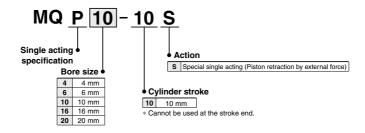
\* The MQP series is not auto switch capable.
