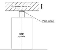
The material of the cylinder rod is heat-treated stainless steel (HRC60). The roughness of the spherical contact of the attaching part (Equipment, Work, etc) should be Rz6.3 and the material should be HB100 or greater (Aluminum material: 2000 line or 7000 line or equivalent) When higher precision or longer service life is required, we recommend using a heat-treated material + flat polished machined material (Rz0.8)
