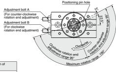
With adjustment bolt, internal shock absorber
