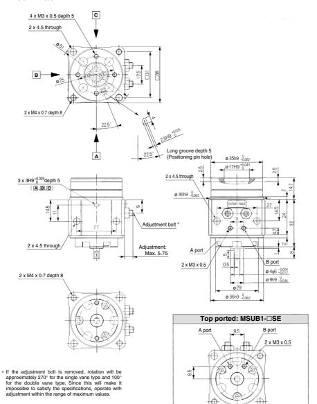
These drawings indicate the condition when the B port is pressurized.
