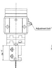
14.7 A port B port 2 x M3 x 0.5 (Port location: Side ported type only) 28 ø 18.5 ø 29
