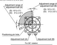
Single vane (S): 80° to 100° adjustable Double vane (D): 85° to 95° adjustable
