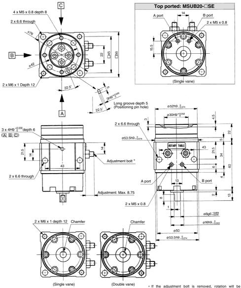
The outside drawings show the single vane type, but only the position of the chamfered sections shown in the above drawings differs from single and double vane.
