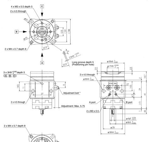
\* If the adjustment bolt is removed, rotation will be approximately 270° for the single vane type and 100° for the double vane type. Since this will make it impossible to satisfy the specifications, operate with adjustment within the range of maximum values.
