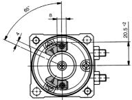
If the adjustment bolt is removed, rotation will be approximately 270° for the single vane type and 100° for the double vane type. Since this will make it impossible to satisfy the specifications, operate with adjustment within the range of maximum values.
