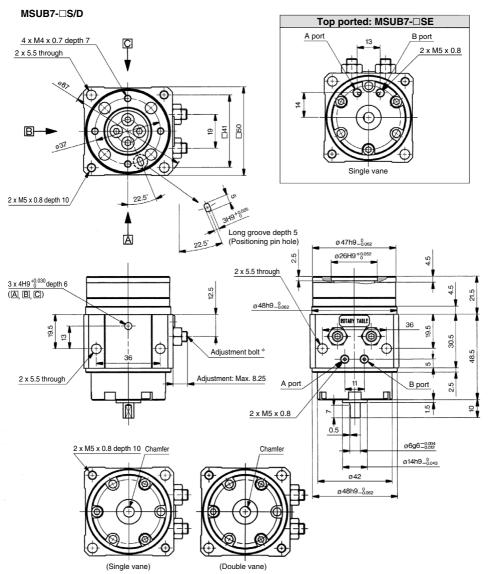
The outside drawings show the single vane type, but only the position of the chamfered sections shown in the above drawings differs from single and double vane.
