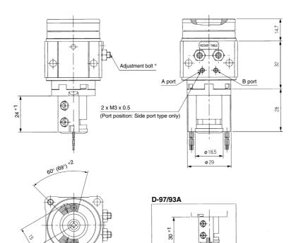
\* If the adjustment bolt is removed, rotation will be approximately 270° for the single vane type and 100° for the double vane type. Since this will make it impossible to satisfy the specifications, operate with adjustment within the range of maximum values.
