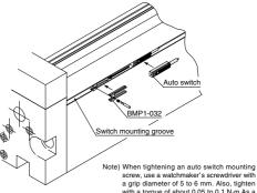
screw, use a watchmaker's screwdriver with a grip diameter of 5 to 6 mm. Also, tighten with a torque of about 0.05 to 0.1 N·m As a guide, it should be turned about 90° past the point at which tightening can be felt.
