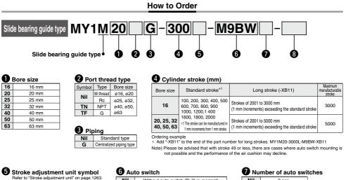
Nil Without auto switch (Built-in magnet) Applicable auto switches vary depending on the bore size. Select an applicable one referring to the
