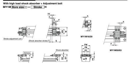
\* Since dimension EY of the H type unit is greater than the table top height (dimension H), when mounting a workpiece that exceeds the overall length (dimension L) of the slide table, allow a clearance of dimension "a" or larger on the workpiece side.
