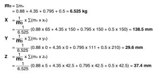
4. Calculation of Load Factor for Static Load
