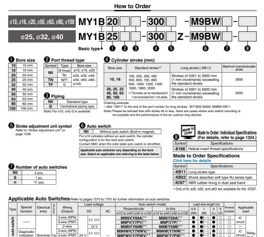
\* Auto switches are shipped together (not assembled)
