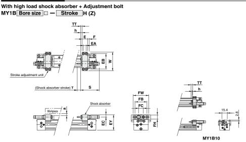
• Since the dimension EY of H unit is greater than the table top height (dimension H), when a workpiece is loaded that is larger than the full length (dimension L) of the slide table allow a clearance of size "a" or larger at the workpiece side.
