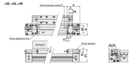
\* Since the EY dimension of H unit is greater than the table top height (H dimension), when a work piece exceeding the full length (L dimension) of the slide table is mounted, allow a clearance of size "a" or larger at the work piece side.
