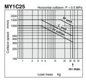
**MY1C50** Horizontal collision: P = 0.5 MPa 2000 unit 1500 s/mu unit 1000 speed 500 400 Collision 300 200 100 3 4 5 20 30 10 40 50 ŧ m1 max Load mass kg
