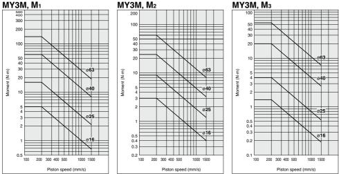
Select the load from within the range of limits shown in the graphs. Note that the maximum allowable moment value may sometimes be exceeded even within the operating limits shown in the graphs. Therefore, also check the allowable moment for the selected conditions. Maximum Allowable Load
