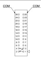
Mixed single and double wiring are available as an option. The maximum number of manifold stations is determined by the number of solenoids. Count one point for a single solenoid type and two points for a double solenoid type. The total number of solenoids (points) must not exceed 24.
