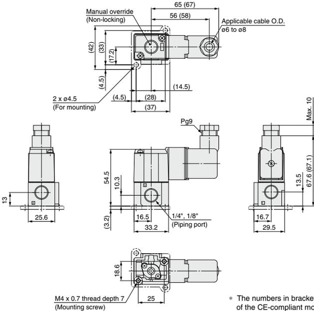
\* The numbers in brackets indicate the dimensions of the CE-compliant model (-Q).
