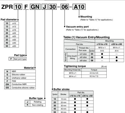
Note) Pads are exclusively ball joint type and are not interchangeable with other pads.
