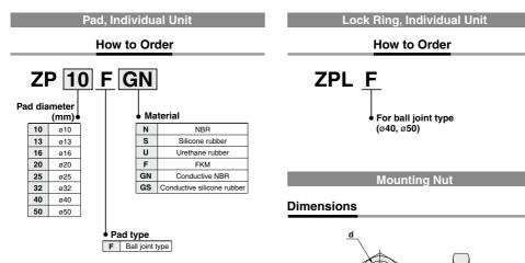
Note) Pads are exclusively ball joint type and are not interchangeable with other pads.
