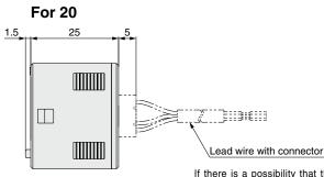
If there is a possibility that the atmospheric vent port of the switch will be exposed to water or dust, insert a tube into the atmospheric vent port and route the other end of the tube to a safe place away from water or dust. (Z/ISE20B)
