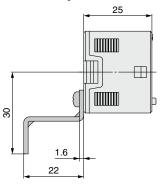
$\ast\,$  When using the bracket B, install it by taking the dimensions of the piping part into consideration.
