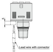
If there is a possibility that the atmospheric vent port of the switch will be exposed to water or dust, insert a tube into the atmospheric vent port and route the other end of the tube to a safe place away from water or dust.
