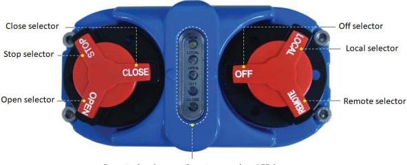
Remote, local, open, Over torque, close LED lamp
