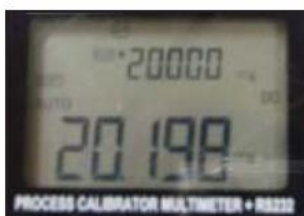
IN/OUT CHECK CLOSE: 4mA, OPEN: 20mA
