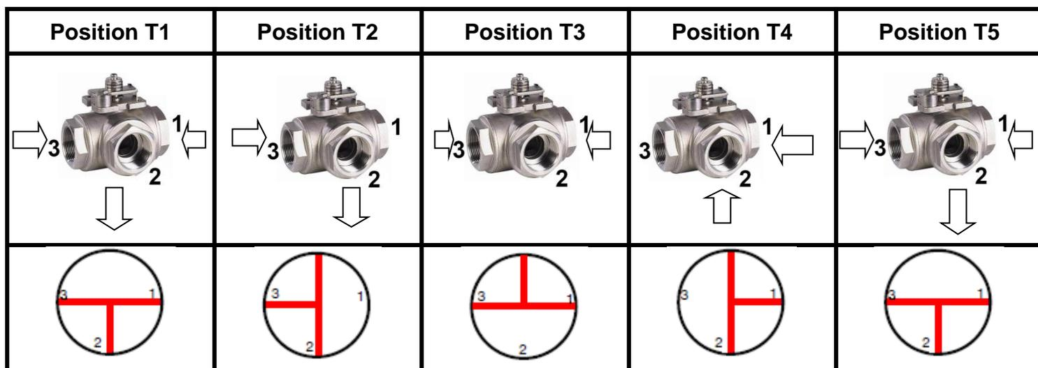
**ROBINET A TOURNANT SPHERIQUE 3 VOIES PN 40 TARAUEE**
