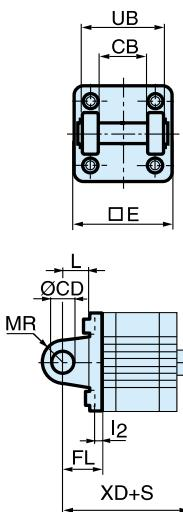
**Compact ISO Cylinders - P1P Series****Dimensions****Cylinder mountings****Clevis bracket MP4**
