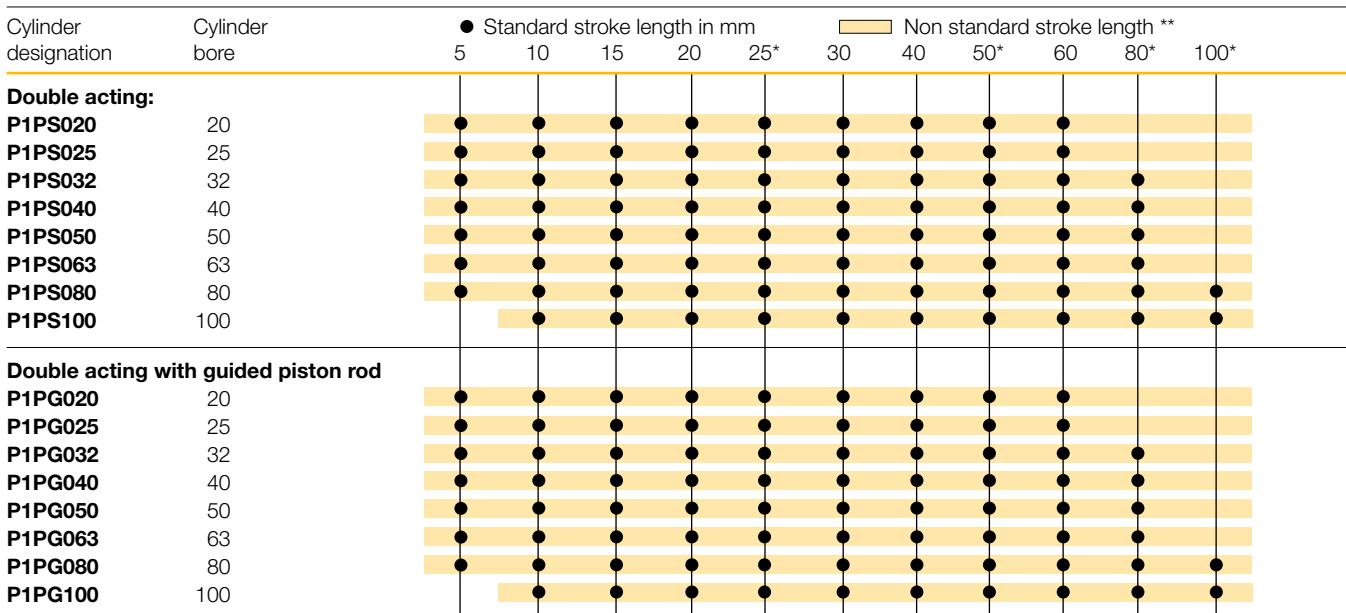
\* Standard stroke lengths in mm according to ISO 4393
