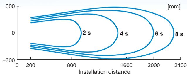
\*1 When neutralising static electricity from 1000 V to 100 V at a distance of 300 mm from the workpiece (front surface). When air flow of IZF31 is maximum.
