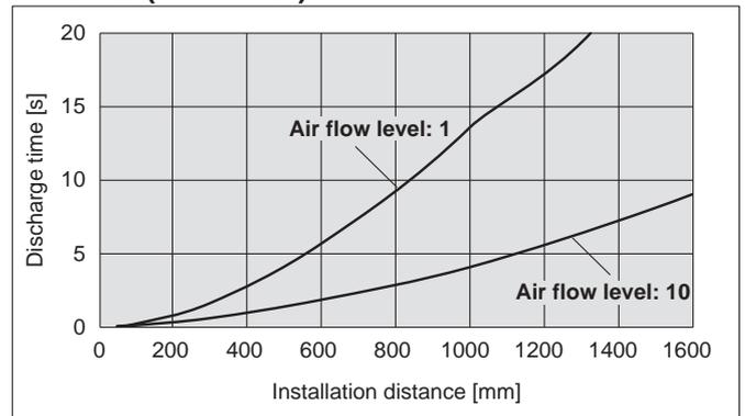
\*: Static neutralisation performance is based on data using a charged plate (size: 150 mm x 150 mm, capacitance: 20 pF) as defined in the EN 61340-5-1: 2007 Standards. Use only as a guideline purpose only for model selection because the value varies depending on the material and/or size of subjects.
