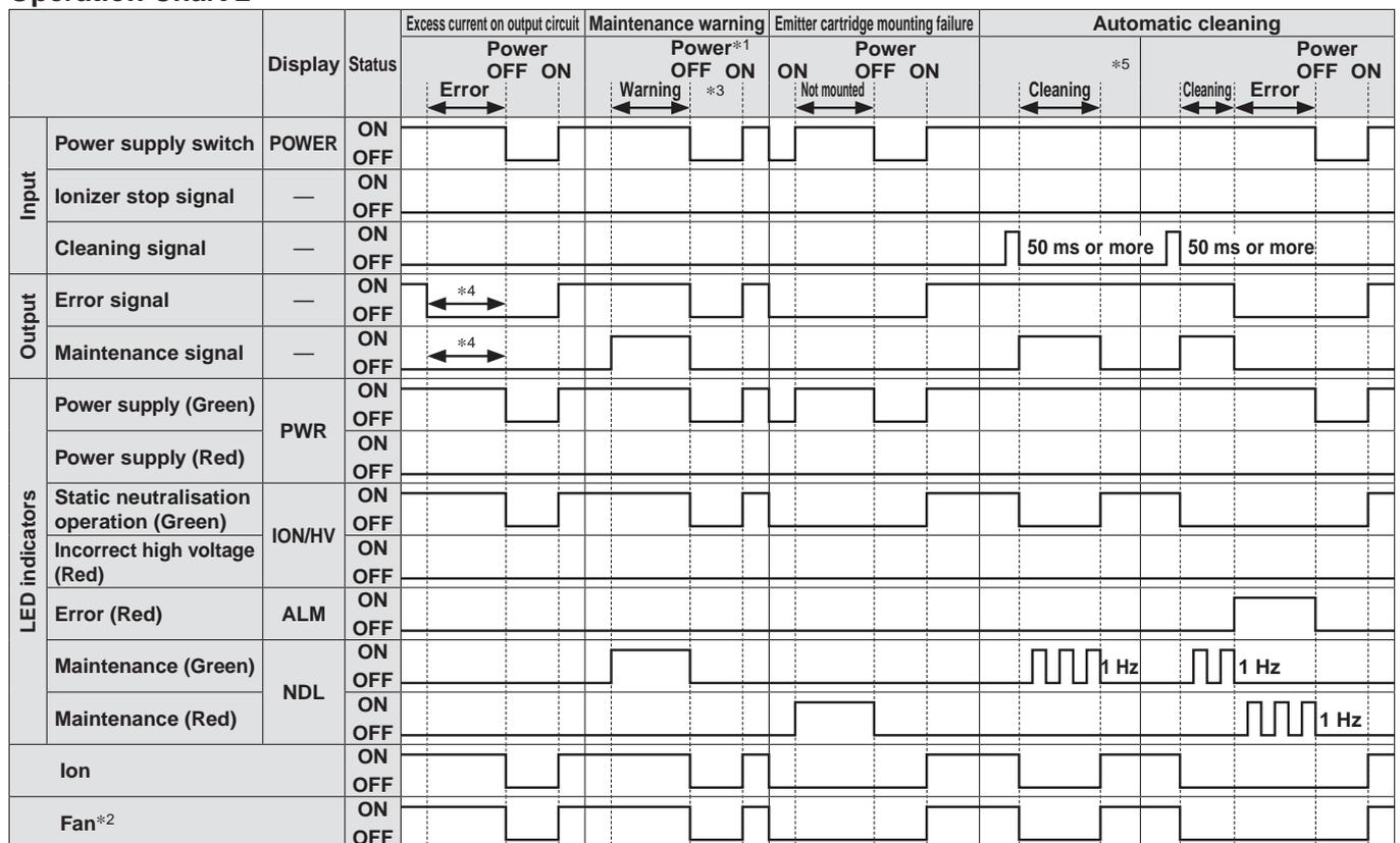
\*1 Incorrect high voltage, fan motor failure, and maintenance warning can also be released by the ionizer stop signal after resolving the error.
