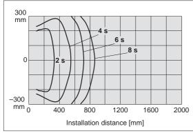
IZF31-W (With adjustable louver: Angle setting 1, Air flow level: 10
