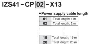
Available in 1 m increments from 1 m to 20 m. Use standard power supply cables for 3 m and 10 m lengths.
