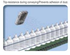
For the static neutralisation of film-molded goods Sticking and scattering prevention on a conveyor
