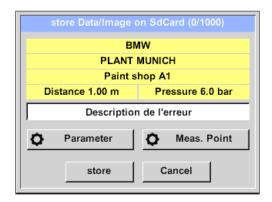
Afterwards it is possible to check the parameters (pressure and distance) and to precisely define the measurement place with company, building and location. It is also possible to enter a short error description (max. 32 characters).
