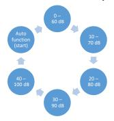
You can manually switch between individual levels with the "Sensitivity" button or use the auto function to adjust the level. The order is shown in the chart on the left.
