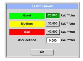
The specific output refers to the efficiency of the compressor system. For example, how much electrical energy (kWh) is required to produce 1 cubic metre of compressed air (m³). Three predefined system values are created for this, as well as a user-defined input field for individual entry.
