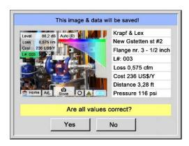
All relevant data of the leakage are shown in the image and a final check can be done again before saving. All leakages, including entries made, are saved to the journal file.
