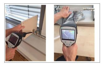
**Superimposition of leaks:** If leaks are close to one another, the emitted ultrasound overlaps. In this case, it is recommended to seal the leakages using a cloth. This enormously increases the accuracy of the measurement, especially for the quantification of the leakage. At the same time, measurements should be taken in close proximity to the components.
