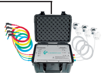
Current/effective power meters
